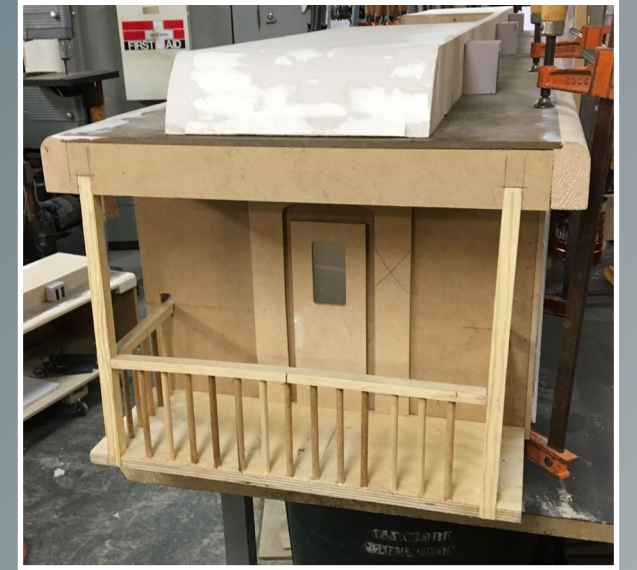
Railing Detail, dowels
